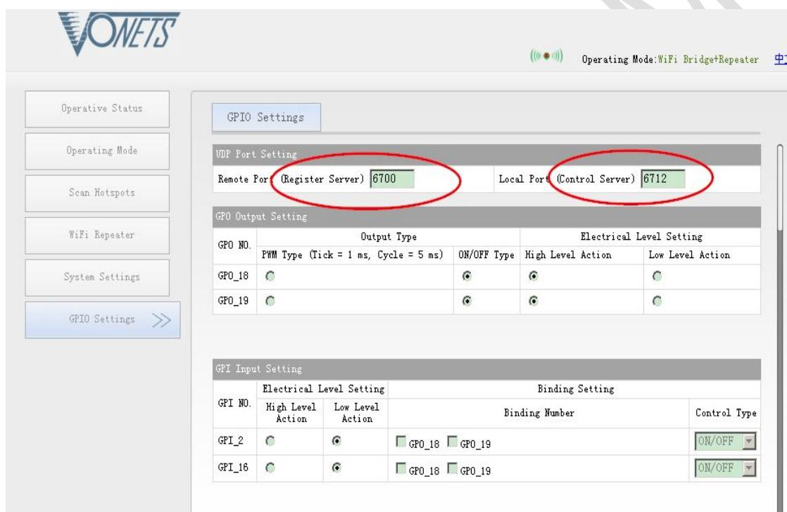
2、 According to the configuration page settings, in VHA300 devices configured correctly GPIO pull up and down the resistance:
