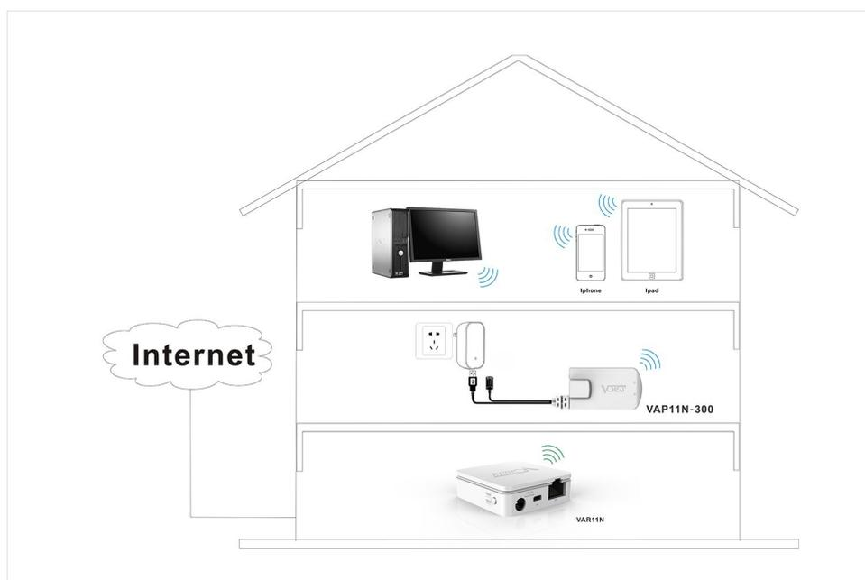
2. Intelligent WiFi Bridge mode(VAP11N): WiFi intelligent bridge function, wireless to wired, wired to wireless intelligent switching.
